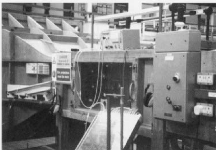
Figure 8 : Pressure bank, velocity control and measurement system of the wind tunnel
