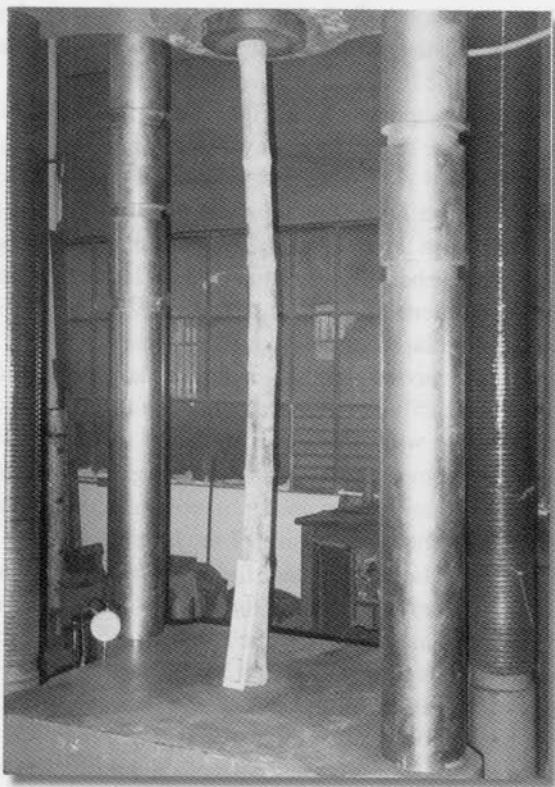
Figure 5 : Testing of full-sized bamboo specimen
