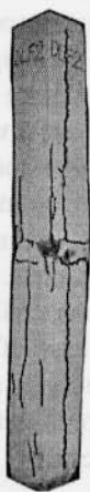
Fig. 5 : Mode of failure and crack pattern of columns with precast ferrocement divided into two halves
