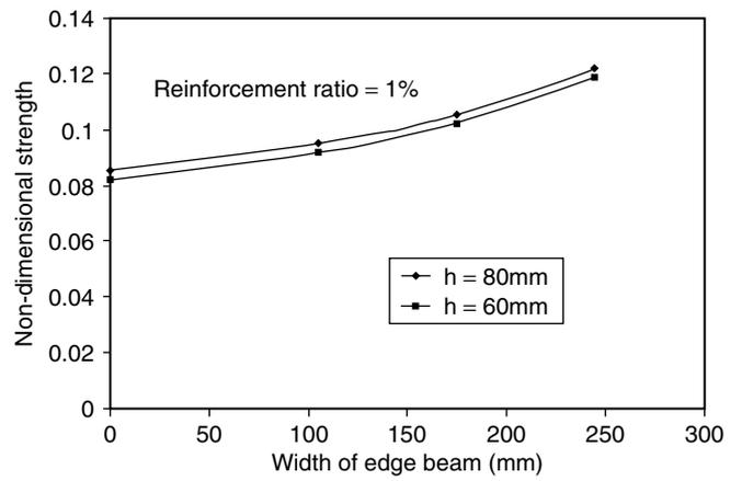
Figure 9. Effect of edge restraint for 1.0 percent reinforcement
