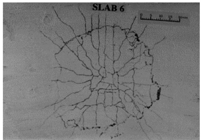
Figure 7. Typical cracking pattern on the bottom surface of a model slab
