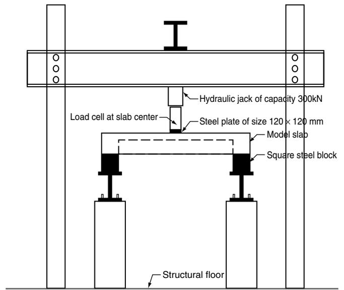
Figure 4. Testing set-up
