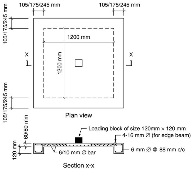
Figure 1. Details of a typical model slab with reinforcement
