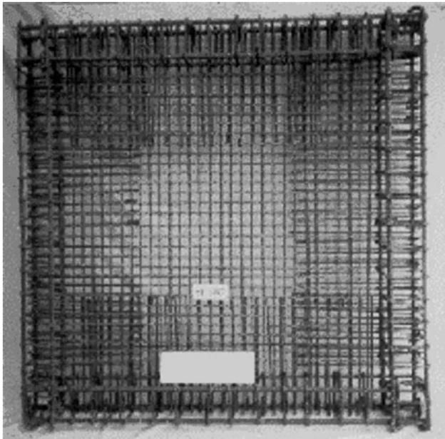
Figure 2. Photograph of typical model slab reinforcement with edge beam
