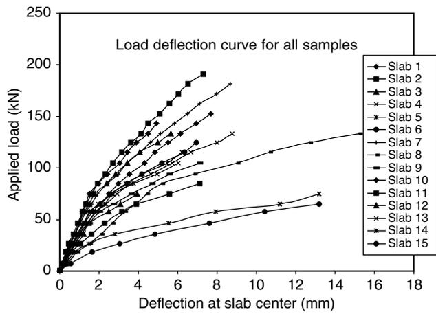
Figure 8. Deflection at slab center of all slabs under different loading
