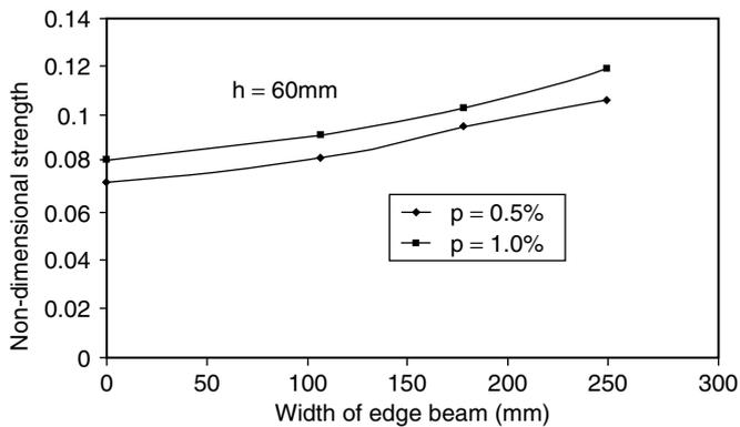
Figure 10. Effect of reinforcement for slab thickness of 60mm
