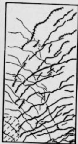
Fig. 2 - (a) Predicted and experimental load-carrying capacities of normal-strength concrete beam C [2], (b) crack patterns in the zone where failure occurred in high-strength concrete beam HSB1 [7], and (c) final crack patterns in repaired shear wall SW 33-R [8]
