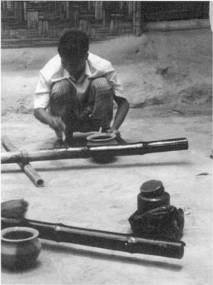
Figure 2.4: Coating Bamboo with Bitumen
