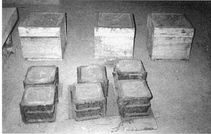
Figure 2.2: Mud Cement Block Preparation
