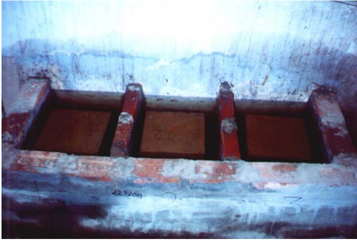
Figure 15: Mud-cement block testing under water
